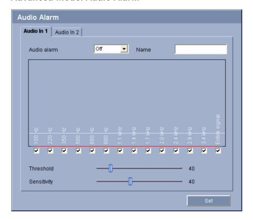
The VideoJet X40 SN can create alarms on the basis of audio signals. You can configure signal strengths and frequency ranges in such a way that false alarms, for example due to machine noise or background noise, are avoided.
